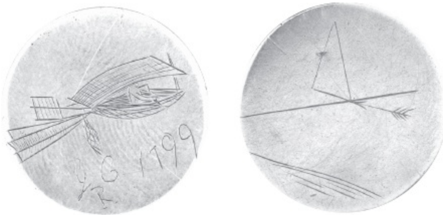
Figure 1.5 The silver disk on which Cayley engraved his concept for a fixed-wing aircraft, the first in history, in 1799. The reverse side of the disk shows the resultant aerodynamic force on a wing resolved into lift and drag components, indicating Cayley's full understanding of the function of a fixed wing. The disk is presently in the Science Museum in London.
